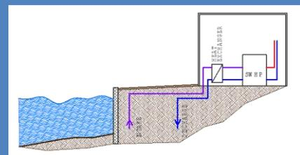
☑ PP # 2 – *Thermal energy - Sea Water Heat Pump with closed loop*
